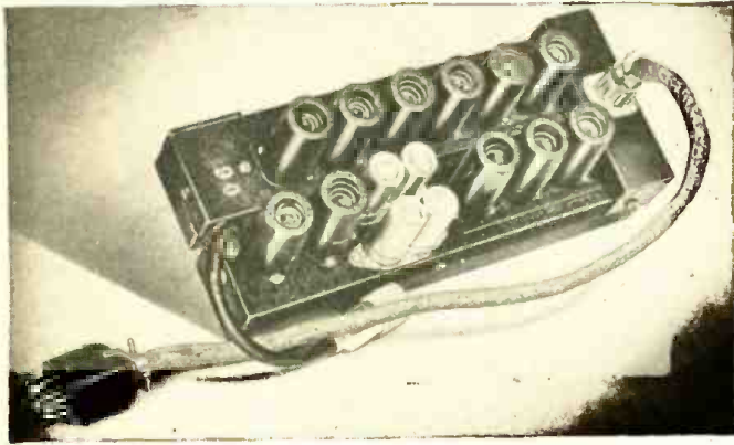
This is the amplifier whose circuit is shown in the diagram below. It does not differ greatly in appearance from ordinary equipment.
